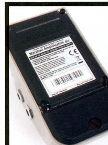
■ Battery access is via the bottom plate: a tiny bit fiddly, but very solid
