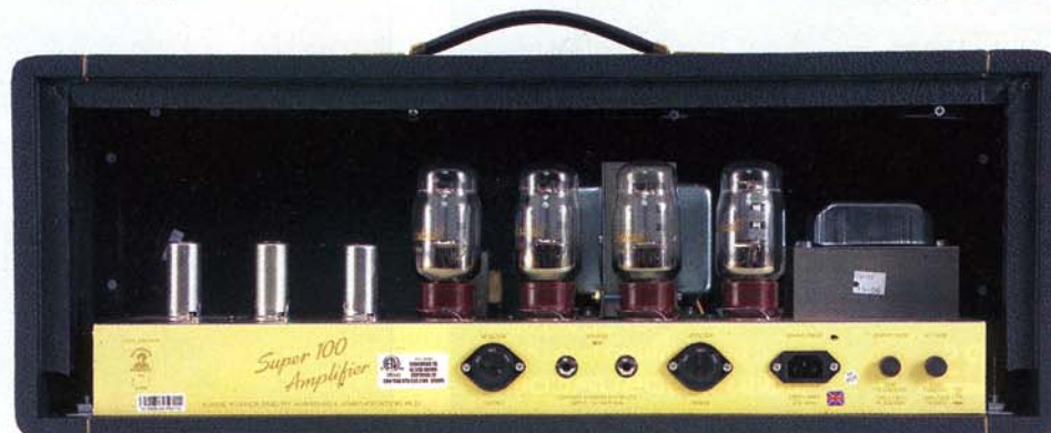
With the rear panel removed, the size of the KT66 power tubes is readily apparent.
