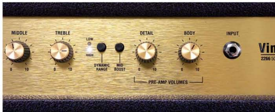
"When the High Dynamic Range is switched in, an extra 12AX7 is added to the signal path," says Vintage Modern designer Steve Dawson. "Both sides of this valve are paralleled for better noise performance. The signal is conditioned to give more available gain and a preset boost, which is optimized to work with the guitar's volume control."
